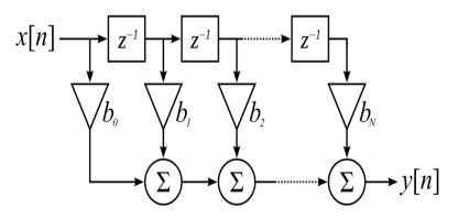
Figure 1: Discrete time filter of order N.
